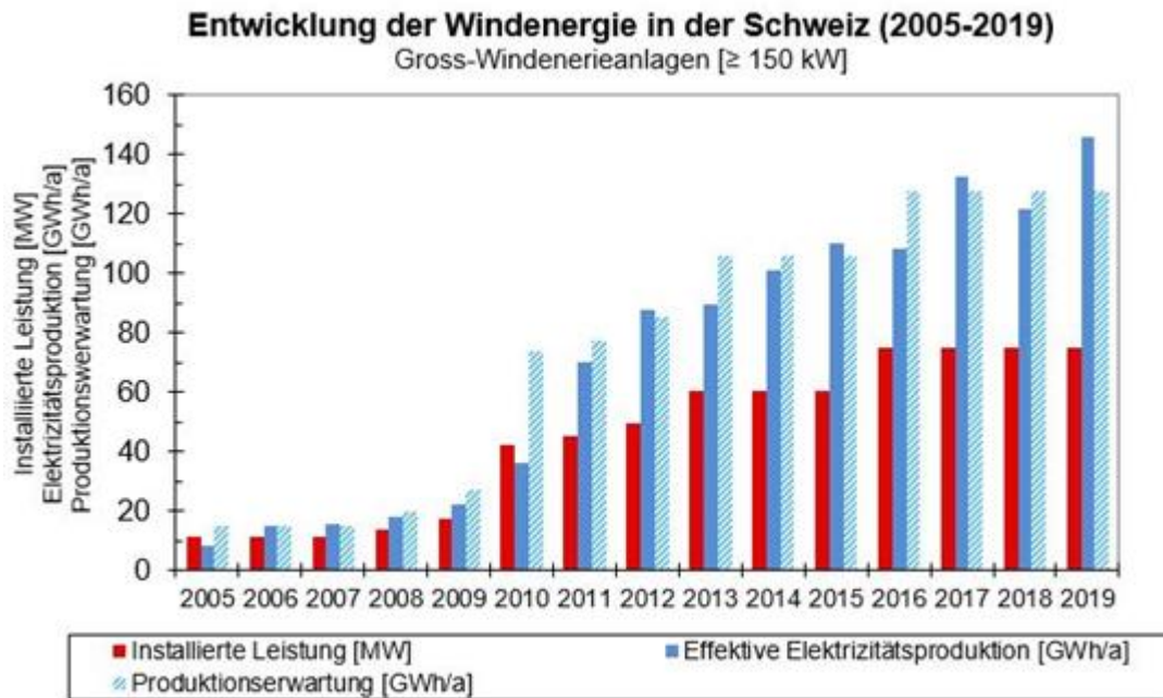
Figure 5-9: The development of the installed capacity (red), electricity production (dark blue) and expected production (light blue) since 2005.
