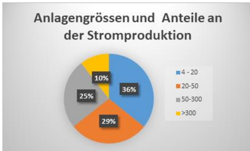
Figure 5-5: Distribution of the electricity yield correlating with the size of the plant according to Table 5-2. Solar plants with a capacity <4 kWp are not plotted because of their minor part in the production of electricity.
